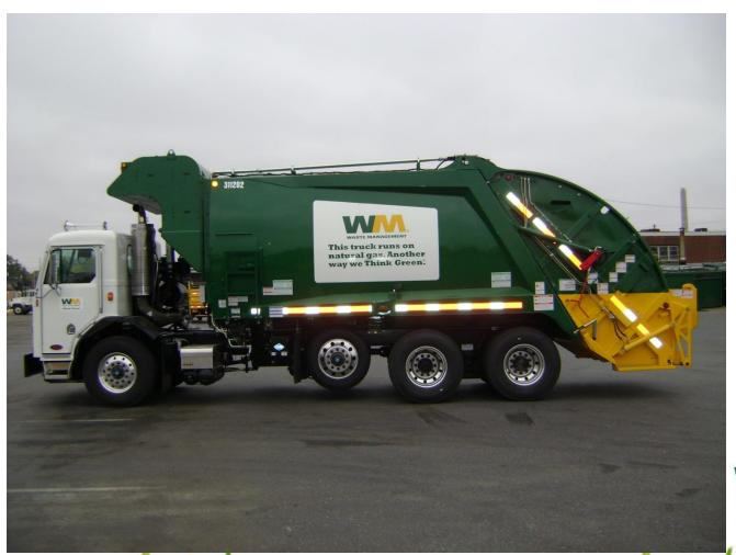
Peterbilt 320 **Cummins ISLG** Engine 330 HP 540 Cu In 1000 lbs torque 75 DGE CNG storage tanks 25 Yard McNeilus Body Rear Ratio 6.14 CNG vs 5.38 Diesel
