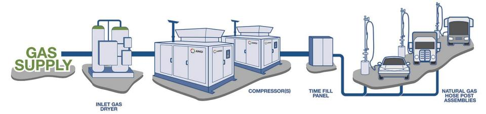
A cost effective fueling option that allows vehicles to conveniently refuel overnight or when the vehicles are not in use.
