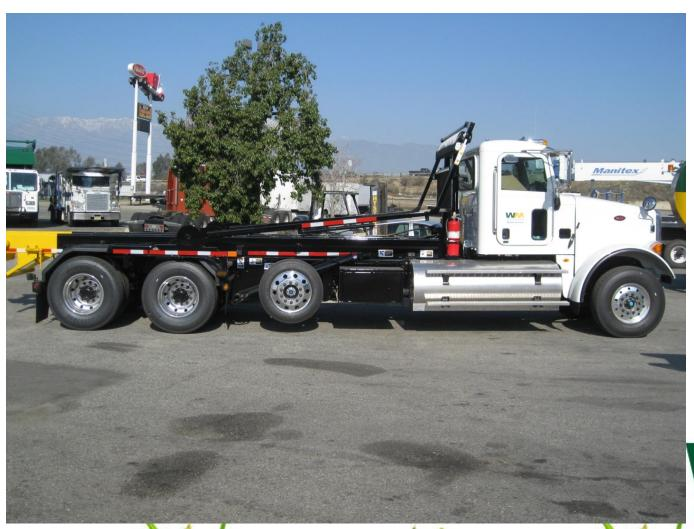
Peterbilt 365 **Cummins ISLG** Engine 330 HP 540 Cu In 8.9 Liter 1000lbs Torque Galbreath RO 75 DGE CNG **Tank Storage** Rear Ratio 6.14 CNG vs 5.38 Diesel
