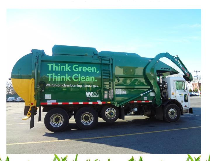
Peterbilt 320 **Cummins ISLG** Engine 330 HP 540 Cu In 1000 lbs torque 75 DGE CNG storage tanks McNeilus 40 Yard Body Rear Ratio 6.14 CNG vs 5.38 Diesel
