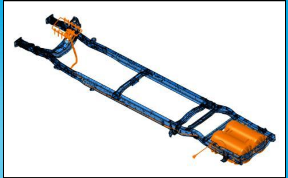
2011 Ford E-450 DRW Cutaway Fuel System
