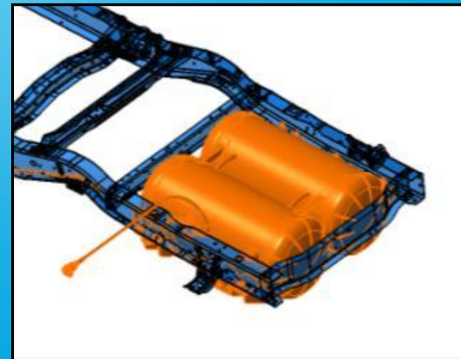
ROUSH CleanTech E-450 Under-Body Tank
